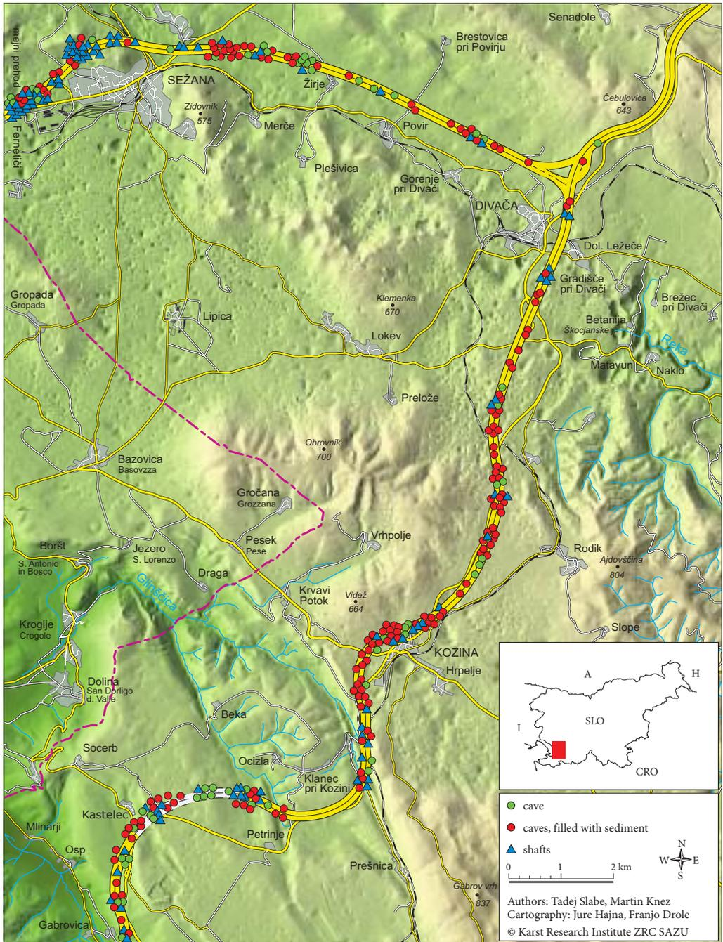
Figure 2: Caves discovered during motorway construction in southwest Slovenia.
