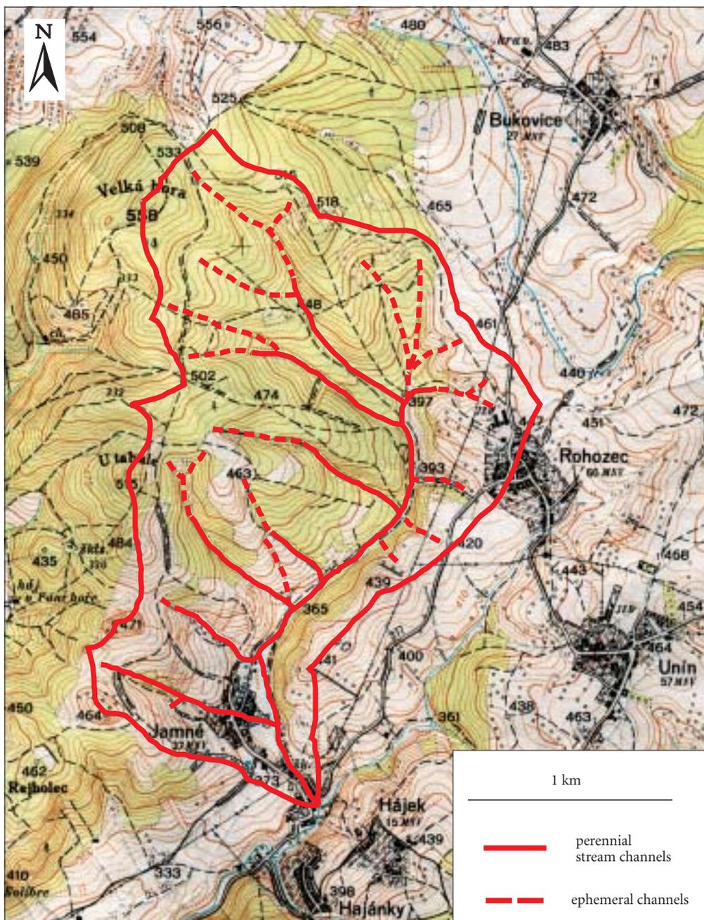
Figure 2: An example of the drainage network delineation from the topographic map 1:25,000 (General map of the Czech Republic, sheet 24-321). The picture illustrates the drainage basin of the third order in the Sýkošská hornatina (highland) bounded with its drainage divide. During the field survey missing dry valleys and gullies are added to the basic skeleton of the drainage network delineated from the map.
